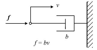
Constitutive Equation: f = bv where b=damping constant (damping coefficient); for viscous damping
