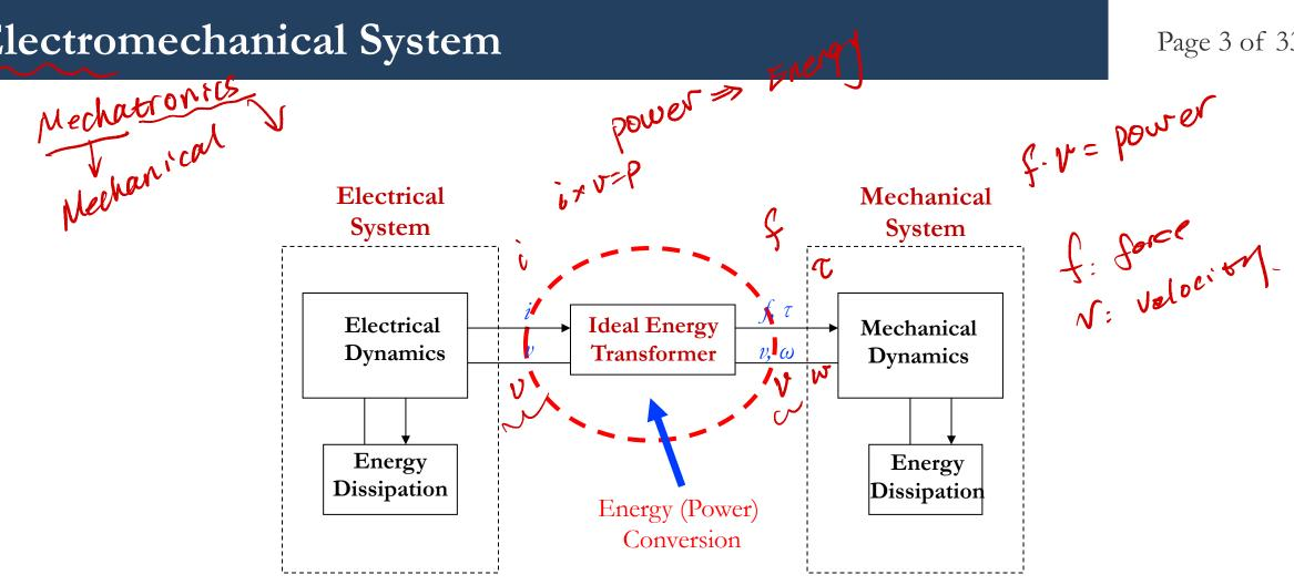
An electromechanical system / mechatronic system
